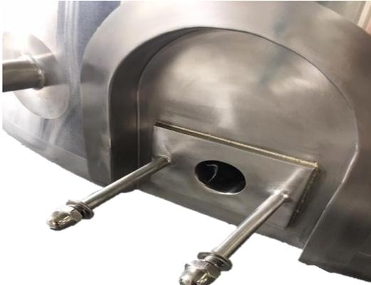
1. Apply Petrol Lube to the gasket and stick it to the base of tank.
