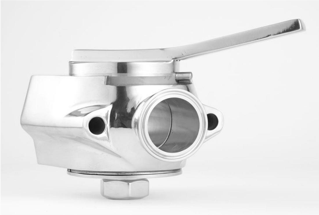
This is stainless steel plug valve. Its close-coupled designed will assure proper heating of product inside valve closure (where the inside wall of vat and valve seat meet). If the valve is not closed correctly; the milk will drip out the valve bottom through the grooves inside the valve cavity. This will prevent raw milk from being allowed back into the pasteurized batch of milk. This valve is required for all legal batch pasteurization and includes a food-grade gasket and Petro-Gel lubricant.
